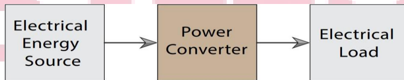
Figure 2: Electrical Power conversion System
